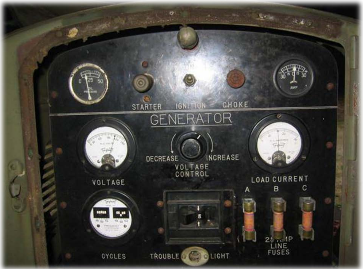
Figure 3 Model 'M5' early 1940's 3 KW genset control panel – note exposed line output fuses. Photo courtesy Phil Waterman
