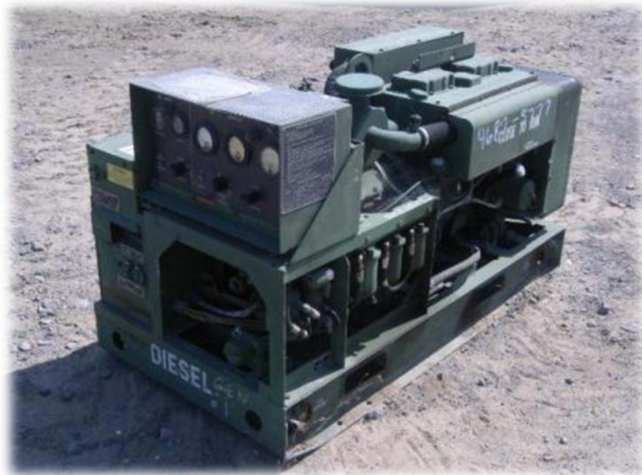
Figure 1 MEP-003A 10 KW Diesel Generator - Photo by Author
